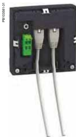
Connection with FDM121 display unit.
